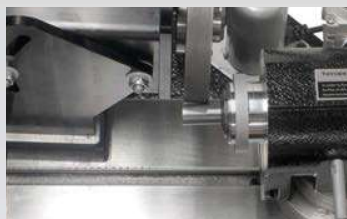
Tapered Weldon Flat Grinding
