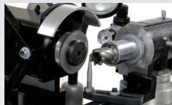
Annular Cutter Sharpening
